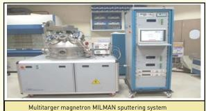
Some of the cermet systems optimized on MILMAN sputter coating system were W-Al $_2$ O $_3$ , Mo-Al $_2$ O $_3$ , W-AlN and W-TiAlN. The best optimised coatings were found as W-Al $_2$ O $_3$  and W-AlN. The optical and high temperature (400°C) thermal emissivity properties for the W-Al $_2$ O $_3$  and W-AlN are shown in the following Fig. 1 and Fig. 2 respectively.
