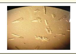
Fig. 1: Plate crystals (PaPVA) formed with tartrate/PEG
