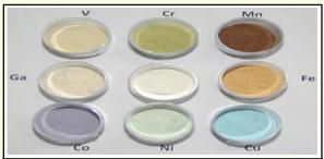
Fig. 3: Photographto show the color associated with different Al<sub>3</sub>GaTM oxides (TM = V, Cr, Mn, Fe, Co, Ni and Cu), Al10Ga oxide (Ga), and the mesoporous  $\gamma$ Al<sub>3</sub>O<sub>3</sub> (center).
