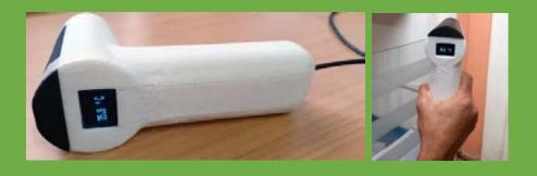
The handheld digital IR thermometer is developed by NCL's Venture Center Incubate, BMek. For the non-contact thermometer, mobile phone or power banks can be used as a power source. Prototype device is currently being used at NCL gate and by Pune Police for screening purposes.
