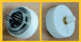
Gauge pressure sensor with SS diaphargm for measuring the pressure range from ±5 kPa to ±100 kPa.
