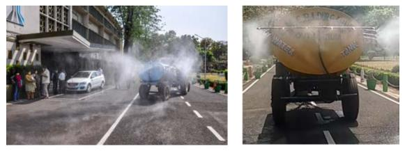
Tractor operated road disinfection spray system
